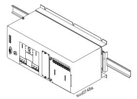
When mounting on the back panel of an enclosure, select screws that are appropriate for the weight of this unit and the mounting surface material.
