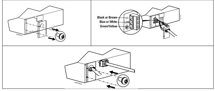
Connect the Battery Modules and Attach the Front Bezel
