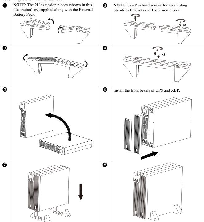
NOTE: Maintain approximately 70 mm distance from the edge of the unit, when installing the stabilizer brackets to the Easy UPS.
