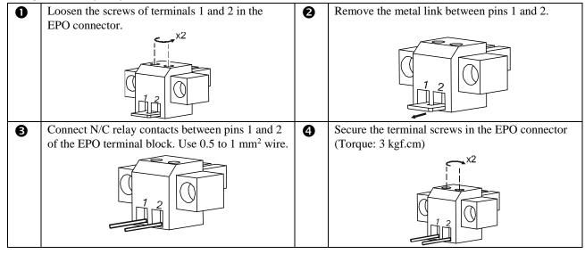
**NOTE:** If the N/C is open, the UPS will turn off and the connected load will not receive power from the UPS.
