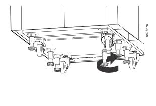
Use one or more levels (not provided) to adjust each foot until the enclosure is level and plumb.
