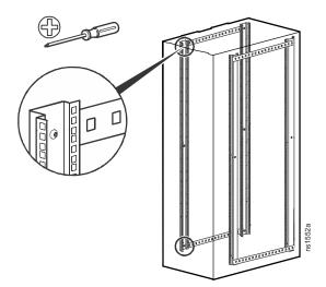
2. Move the pre-installed caged nuts to the desired location, then reposition the vertical mounting flange to this position and install the screws.
