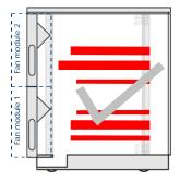
Each fan module has a triangular metal section which protrudes slightly into the enclosure. This does not create an issue for installation of most equipment, but to allow for ample cabling space to the rear of the enclosure, deep servers should be installed in the enclosure space above and below these triangular metal protrusions.
