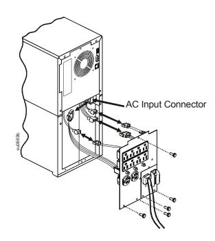
Secure the replacement input and output panels (supplied), to the UPS. Secure the panels with four of the screws removed from the factory installed PDU panel.
