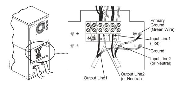
Connect the terminal block and UPS connectors as shown in the diagram.
